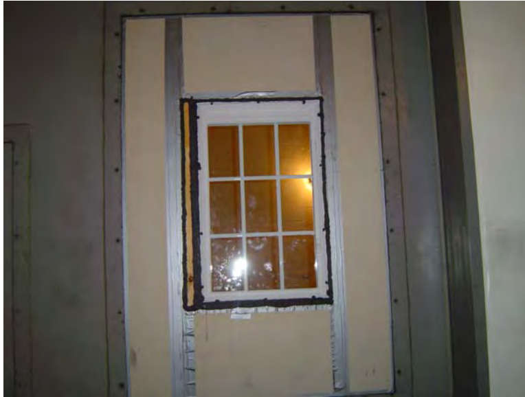
Interior of Sample Installed in Test Opening (Blinds Raised and Stacked)
